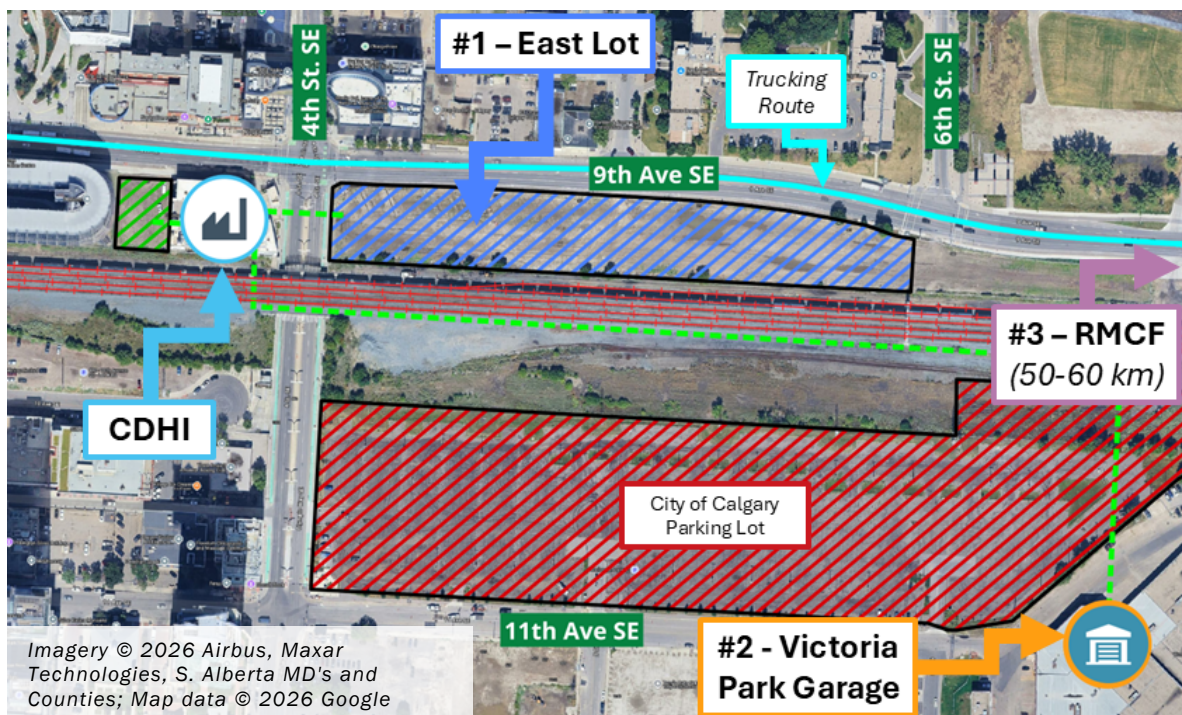
Figure 6 Potential pipeline-based hydrogen supply locations near CDHI
