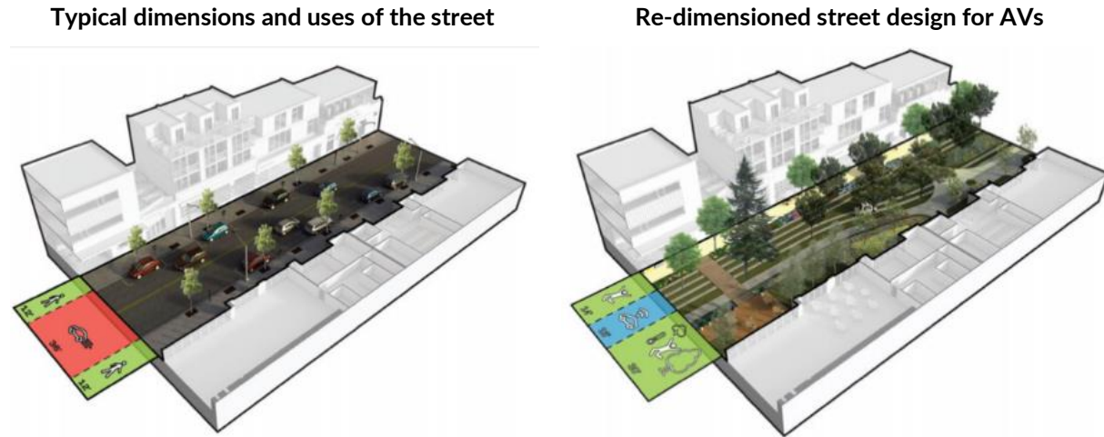
Figure A.8 How Autonomous Mobility on Demand (AMoD) could impact road and streetscape design. [48]
