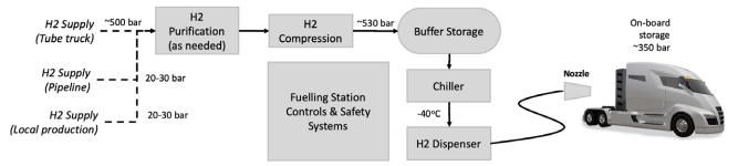
Figure 4.1. Gaseous Hydrogen Fueling Station Configuration. Adapted from NREL [69].
