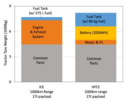
**Figure 2.1.** Estimate of Vehicle Tare Weights for Hydrogen Fuel Cell Electric and Diesel Internal Combustion Heavy Duty Vehicle travelling 1000km with a 17 tonne payload. Analysis completed by CESAR with assumptions supported by literature [16], [29]– [31]; Fuel efficiencies of 2.2  $L_{diesel}$  /100km and 8 kg<sub>H2</sub>/100km assumed.
