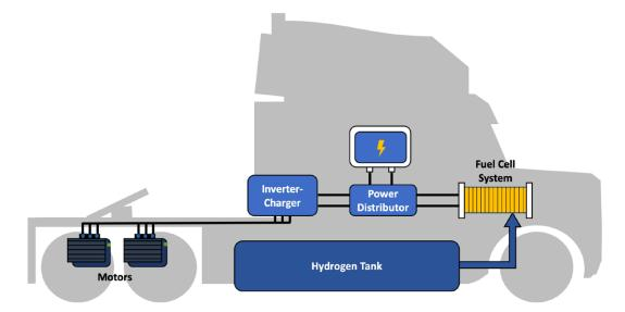
**Figure 1.2.** Example Configuration for a Hydrogen Fuel Cell Electric Heavy-Duty Truck. CESAR figure adapted from Mojtaba Lajevardi et al., 2019 [18].
